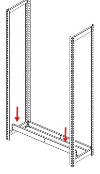
**6.** Attach the remaining shelf supports at the desired shelf levels, making sure that all shelf supports are completely seated in the upright slots.
