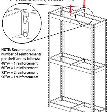
**8.** If particle board decking (Ref. No. 6) or wire decking (Ref. No. 7) was ordered, place the decking on each shelving level. The decking should fit flush inside the shelf supports. If you have purchased a single unit, your shelving unit is now complete. For adder units, see step 9.
