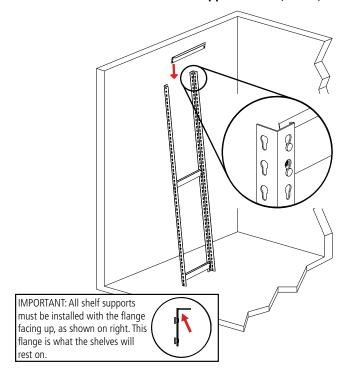
**4.** Place a third front-to-back support in the middle slots of the two uprights (at the level you want your third shelf to be). This forms one end of the shelving unit. Repeat steps 3 and 4 to construct a
