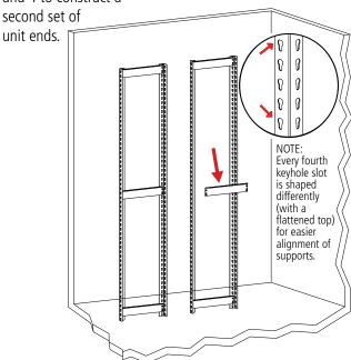
NOTE: If you are planning to install an adder unit, this second set of uprights should consist of ZTP uprights (Ref. No. 2) to act as an intermediate assembly. Carefully review step 2 to better understand.
