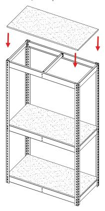
**9.** If joining more than one unit together, your original unit should have been assembled with ZTP uprights on one end, as described in step 4. Simply continue adding shelf supports and uprights to complete your additional units.
